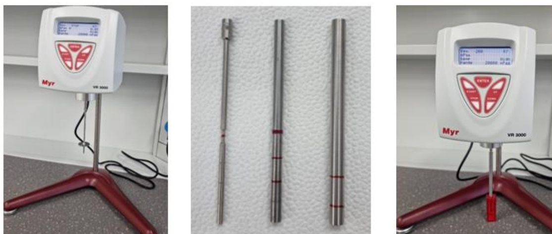
Figure 1. (Viscometer Myr VR 3000; additionally, manufactured spindles; determination of viscosity under standard conditions in a foil-insulated vessel.)
