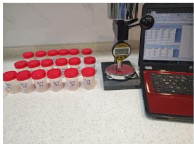
Fig. 6 shows the use of a Sure D device to measure microhardness.
