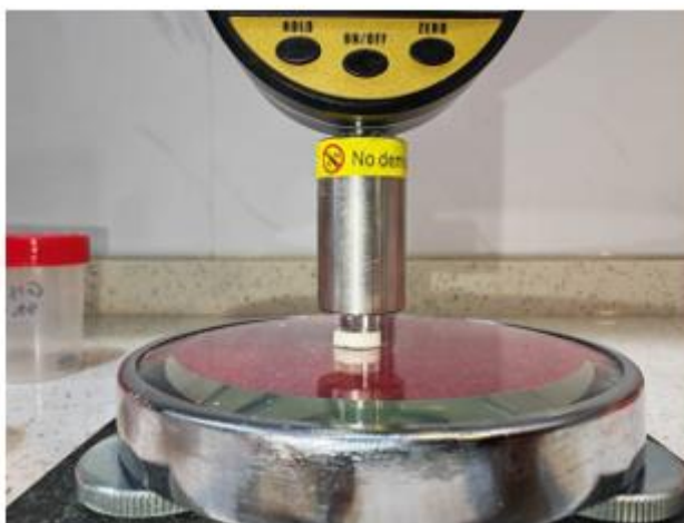
Fig. 6 shows the use of a Sure D device to measure microhardness.
